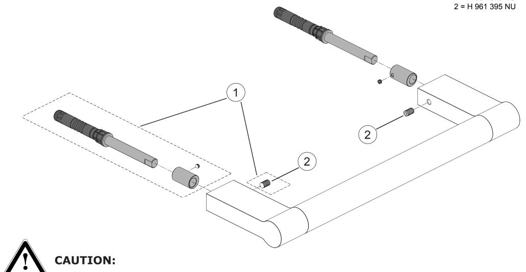
Mounting kit for fixing to the wall provided with this product for applications on solid structures (example: brick or concrete walls).
